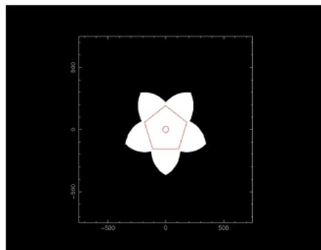
The *white* areas indicate the regions where showers would trigger an array consisting of two concentric cells, each having 5 telescopes.
