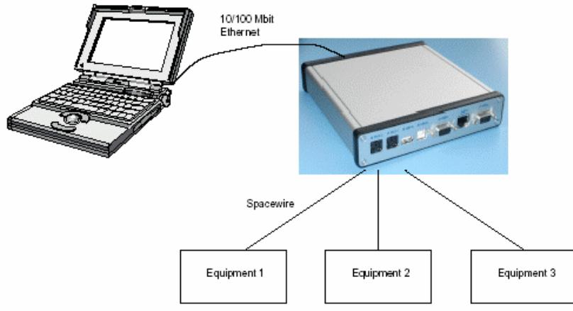
Figure 1. GRESB system diagram
