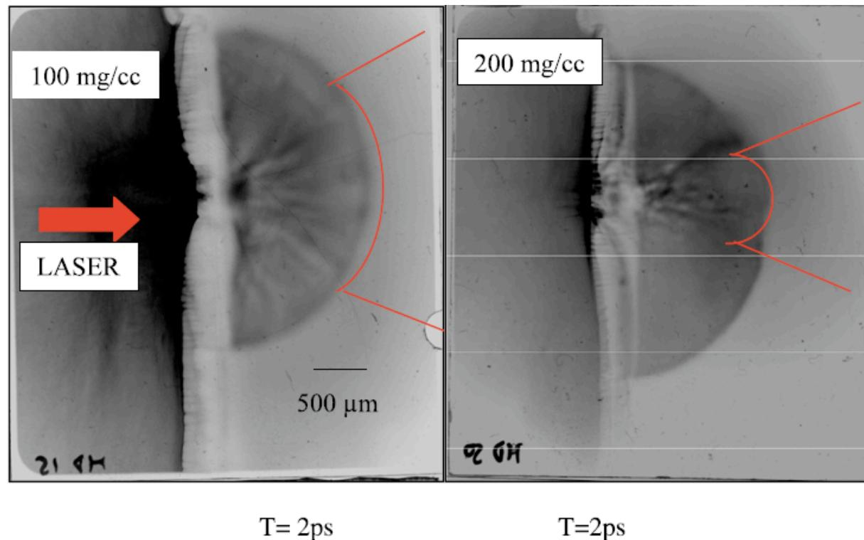
**Fig. 3** RCF images of foam targets following CPA interaction. The density of the foam is indicated in figure. Timing relative to the interaction is indicated below the figures. The hemi-circular shadow on the right side of the images is due to the half-washer enclosing the foam (see Fig. 2), while the *vertical white band* at the centre of the images
