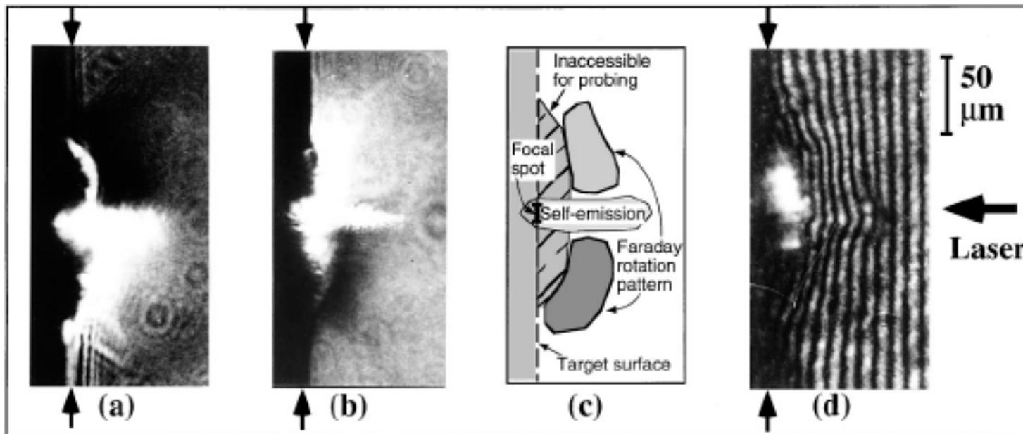
FIG. 1. (a), (b) Polarigrams taken 12 ps after the interaction of a 10 TW, 1.5 ps laser pulse with a solid Al target, with the two polarizers  $-9^\circ$  and  $+12^\circ$  off crossed. The position of the target surface is indicated by the arrows. (c) Schematic showing the main features of the polarigrams. (d) Interferogram recorded 15 ps after the interaction.
