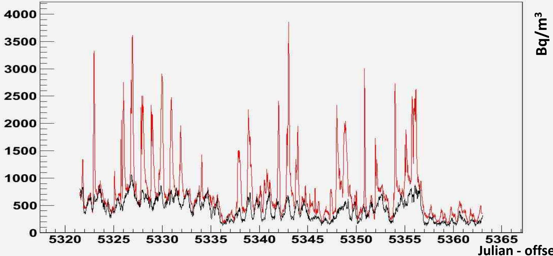
Radon enters the Argo hall from soil and cracks ,mainly on the north side (impressive concentration!!!) and exit through doors and windows with an ease dependent on ventilation and atmospheric conditions
