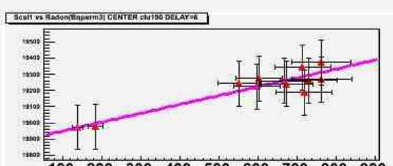
FIT Delay 3h – Radometer@carpet center – Press. cut 602mbar
