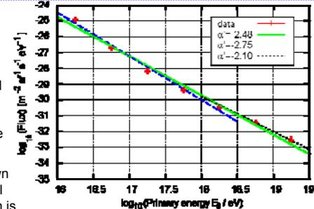
Fig.6 The primary energy spectrum obtained by the OUS1.
