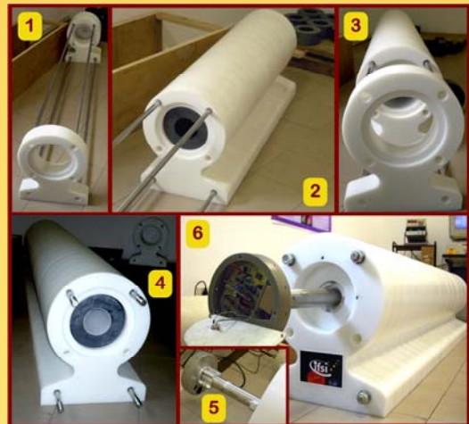
Fig. 2. Step by step assembly of the new modular Cosmic Ray detector.
