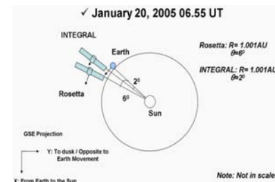
Figure 7. Positioning of the INTEGRAL and Rosetta satellites on January 20, 2005 with respect to Sun-Earth line
